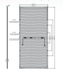
\* The unmarked tolerance is ±1 mm Length shown in mm
